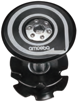
RS-3228 Material:AL6061 CNC Bolt : Stainless Size : 1-1/8" Weight : 26 g
